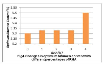
From the above figure it is clear that optimum bitumen content is increased from 5.3% to 5.33%, when RHA is added as filler into the mix upto 3%. The optimum bitumen content is further increased to 5.5% with the addition of 4% RHA into the mix.
