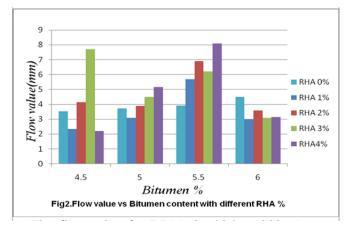
The flow value for DBM should be within 2-4 mm according to MoRTH. From the above figure it is clear that the samples, apart from those which are prepared with 5.5% bitumen, are showing better results than conventional mix.
