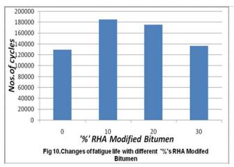
From this figure it is very clear that the fatigue life of conventional mix is increased by about 44%, when 10% and 20% RHA modified bitumen is used. The fatigue life of the sample prepared with 30% RHA modified bitumen is somewhat similar to the conventional sample.
