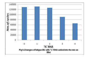
From the above figure it is clear that the fatigue life of the samples prepared with 1% and 2% RHA, added as filler, is more or less similar as comapred with the conventional mix [0% RHA]. The samples prepared with 3% and 4% RHA are showing lesser values of fatigue life.
