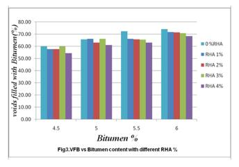
The VFB values should be within 65%-75% for DBM mixes as per MoRTH. From the above figure it is clear that the samples apart from those prepared with 4.5% bitumen is satisfying the criteria as specified by MoRTH.
