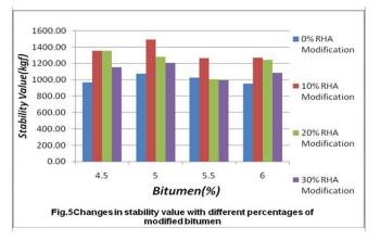
From the above figure it is clear that the samples, prepared with 10% and 20% RHA modified bitumen, with every percentages of bitumen, is giving much higher stability value as compared to the conventional mix [0% RHA Modification].
