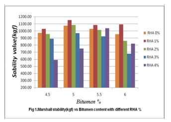
The minimum stability value for DBM mixes is 900kgf as per MoRTH. From the above figure it is clear that the addition of RHA by 1% with every bitumen percentages has given the better stability value as compared to conventional mix [RHA 0% in Fig.1]. Also the addition of RHA up to 2 % into the mix is giving more or less similar results as conventional mix.
