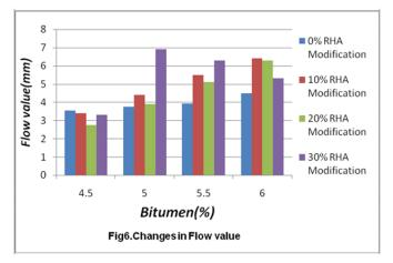
Although 10% modified bitumen is giving better result than the rest. With 30% modified bitumen, the stability values are more or less similar to the conventional mix.
