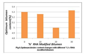
From the above figure it is clear that the optimum bitumen content gets reduced for the mixes prepared with 10% and 20% RHA modified bitumen. For 30% RHA modified bitumen the value is higher as compared to the conventional mix.
